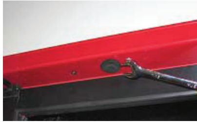
Figure 9 Remove Hold-Open Bolt
