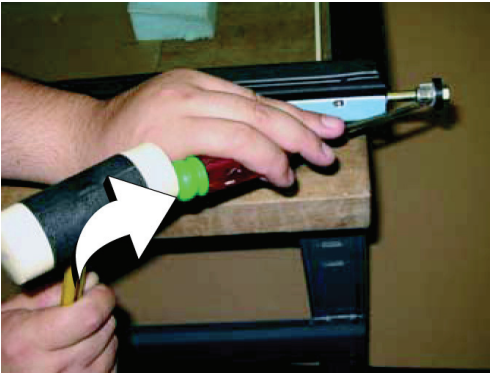
Figure 19 Remove Torque Rod
