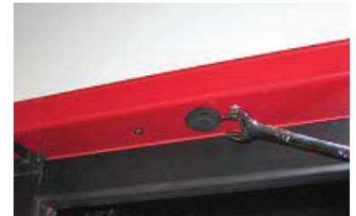
Figure 7 Tighten Hold-Open Bolt
